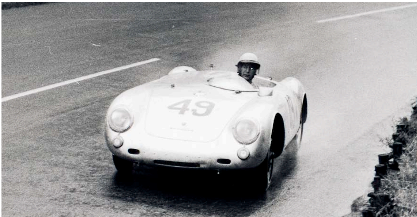
Above: The lightweight aluminium-skinned body of '0048' showing off its front-brake cooling intakes as they gulp in rain and spray during the long 24-Hour grind.
